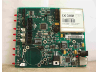
GSM/GPRS Base Station
